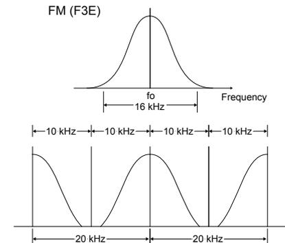
The regular FM mode occupies 20 kHz that is a double the bandwidth of D-STAR.
