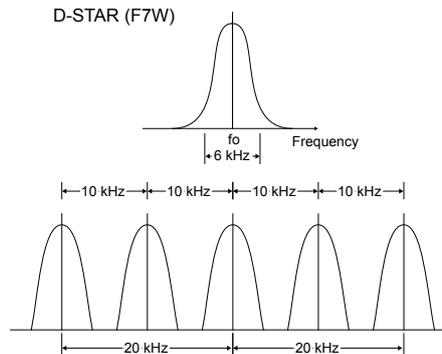
D-STAR operates in 10 kHz steps. The sound quality is good, even though the bandwidth is half of regular FM mode signals.
