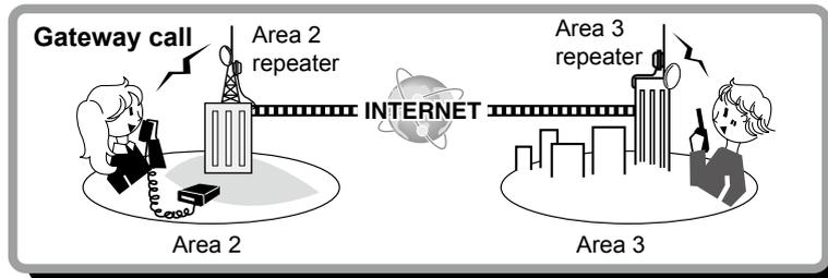
To call through your local area (access) repeater, repeater gateway and the internet to your destination repeater or individual station's last used repeater, using call sign routing.
