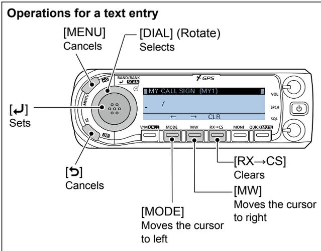
**TIP:** You can enter a note of up to 4 characters, such as the model of the transceiver, name, area name, and so on, after your call sign.
