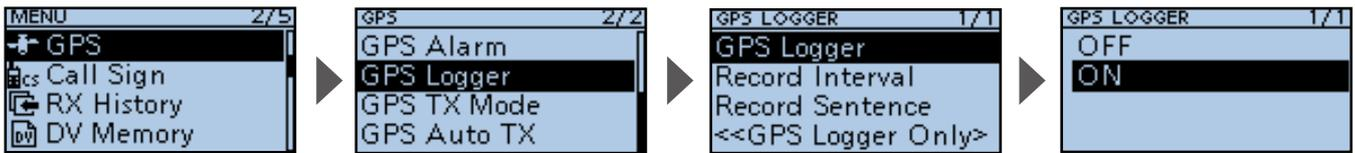
**NOTE:** When using an external GPS, only the supported sentence is recorded among GGA, RMC, GSA, and VTG.
