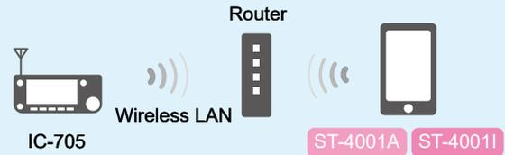
① The IC-705 (firmware version 1.20 or later) can directly connect to your mobile device as a wireless access point.
